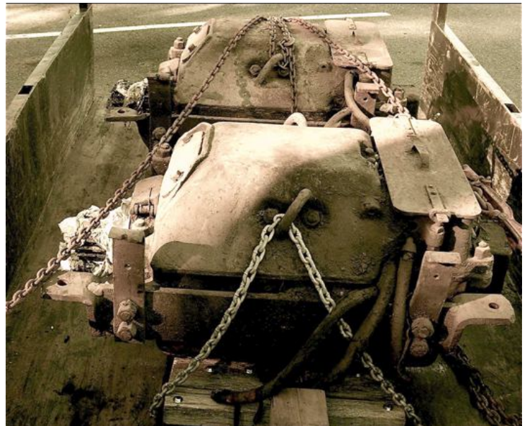
The two traction motors, chained down on a heavy-duty trailer and on their way to Maine for complete overhaul - a round-trip that kept Dave Dye and Sam on the road for 17 hours.
