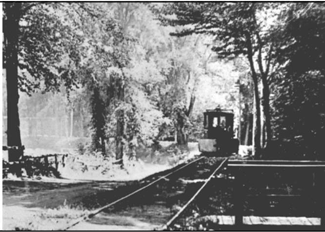
While not appropriate to the season due to lack of snowfall, here is a view of SF&C Plow No. 24 near the Grisworldville canal. No. 24 was a 4-wheeled car which could do light duty as a freight motor.
