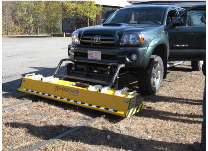
HyGround's subgrade testing rig on SFTM's main line.
