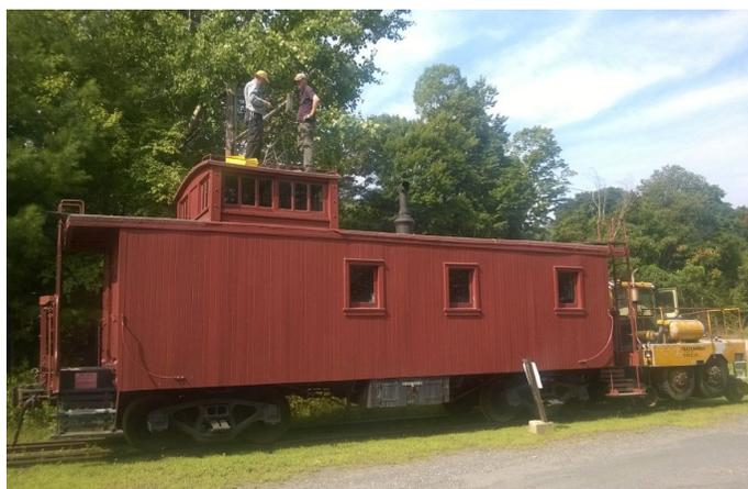
*Nash, Dave and Sam perform preventative maintenance on the bracket arm that holds the trolley wire at Pole 4. Caboose CV4015 and the 9TM Trackmobile assist.*
