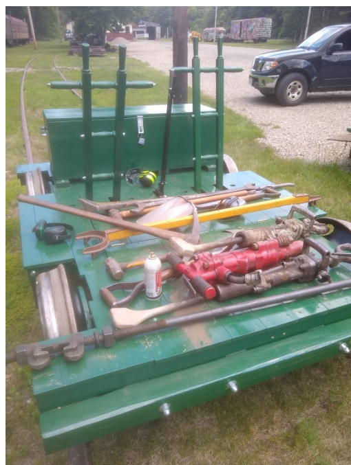
Josh built this handy track car. Here it is being put to use hauling our heavy track tools.
