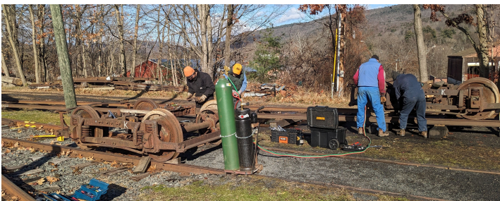
Josh, Martin, Nash and John work on the trucks for the Berkshire Hills
