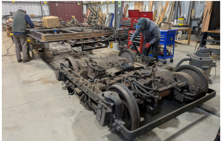
One truck has been rolled out for better access
