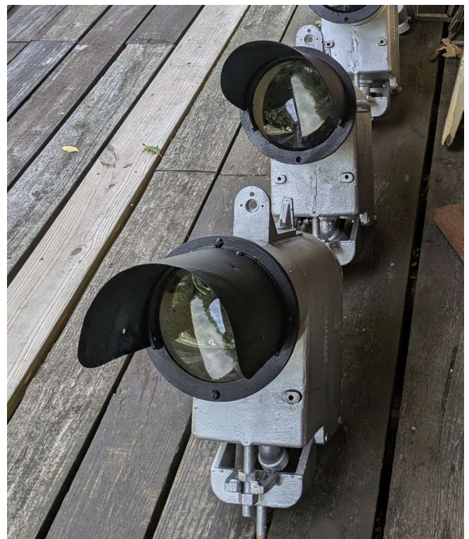
Below: Signal heads ready to be installed
